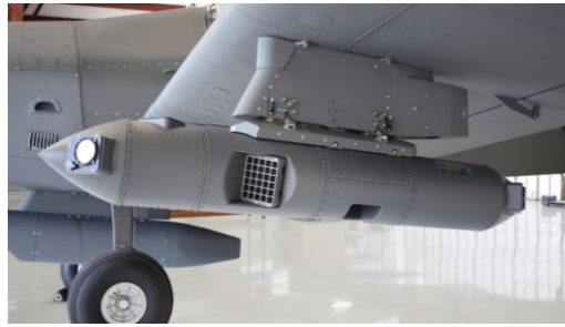
Archangel MWS/CMS Pod
